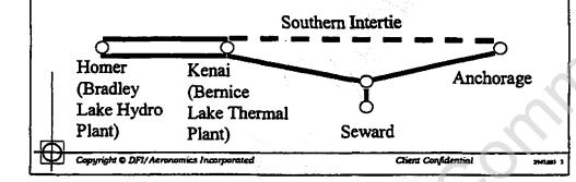
Just to review, the Southern Intertie is designed to provide an alternative transmission routing between Kenai and Anchorage. There are already two transmission routings available between Homer and Kenai.
